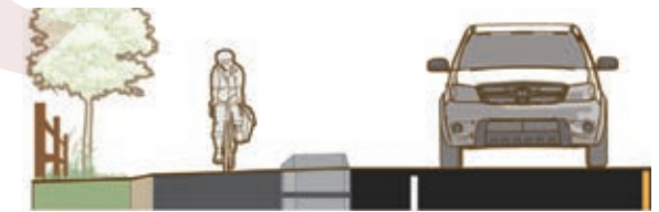
Figure 4-19. Separated bike lanes may be configured on an existing roadway surface by using a physical barrier such as a curb or median to separate the bikeway from the roadway.
