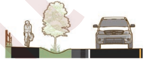
Figure 4-18. Separated bike lanes may be separated by an unpaved roadway separation, and a vertical element. When configured as directional facilities, separated bike lanes should be provided on both sides of the roadway.
