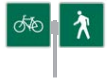
Figure 4-21. MUTCD signing options for specifying user types and path positioning can be used to indicate which users belong on the separate parts of a separated bike lane corridor (D11-1a, D11-2).
